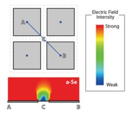
**Figure 2a:** Conventional square pixels with corresponding electric field intensity
