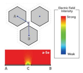
**Figure 2c:** Fujifilm's hexagonal pixels with corresponding electric field intensity
